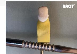
4. Vibrate to minimize the shrinkage
