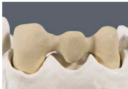
After firing, VINTAGE PRO Opaque should have a non-transparent, silky-matt surface. The framework should be completely masked by the opaque.
