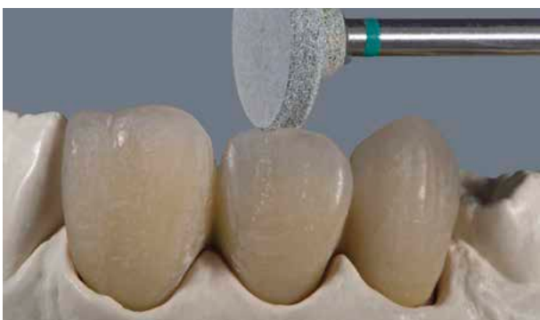
The gloss level is increased in specific areas by prepolishing with silicone polishers.
